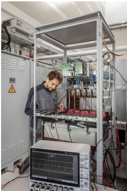
Design and testbench of SiC inverter stacks in the laboratories of Fraunhofer ISE ©Fraunhofer ISE
